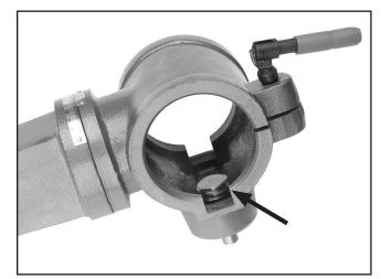
Figure 7. Pinion correctly installed in table support.
